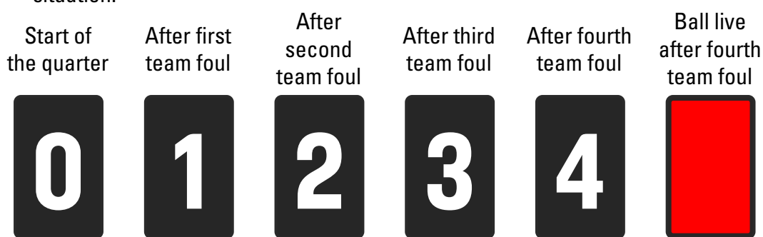
Diagram 12a Electronic team foul marker (example of the layout)
